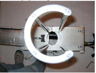
Safety Ring Guard shows the projection of the throwing arm when in use to ensure safety. TO ASSEMBLE:
