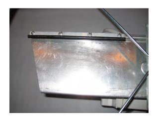
Because the clay lands directly onto the throwing arm, the White Wing needs little adjustment. Loosen the two bolts on either side of the trap to adjust your throwing angle. Once desired angle is reached, tighten bolts back.
