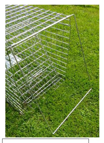
At the front and the middle of the trap there is a support barwhich will stop the cage from folding. Fold the bar and tuck it underthe base of the trap
