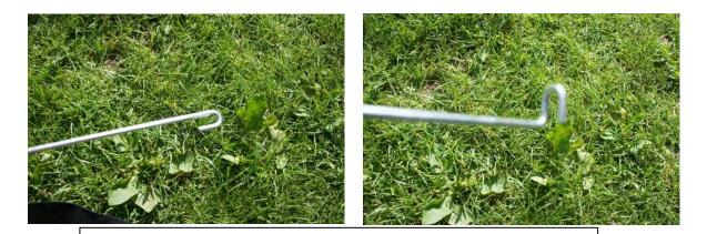
Supplied with the fox trap is a long metal rod with 2 hooks as shown in the photo, the U bend hook in the right photo hooks through the metal plate inside the trap, the hook to the left hooks onto the spring clip as shown in the below picture. The rod hooks onto the u bend spring clip whilst the L shape metal hook goes onto the door whilst in the cocked position.
