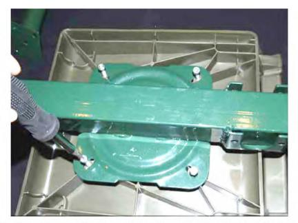
If not already attached, secure the seat to the seat post with the 4 self tapping screws.
