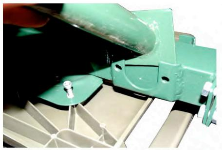
Take the four support legs and slot the into the leg brackets as per pictures. Note that the predrilled hole at the end of each leg are the feet not the mounting brackets. Therefore, The square plate with the hole should be the end that will be sitting on the ground. Now you're ready to attach the trap head. (separate instructions)
