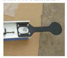
Place the paddle-shaped counter balance on the arm, aligning all pre-drilled holes. By using the allen screws, attach the throwing arm and counter balance to steel mounting plate and secure tightly with provided allen wrench.
