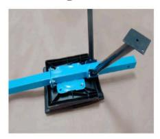
Take plastic seat and position onto the seat plate/seat assembly making sure the seat back folds toward the flat mounting plate for the tail beam assembly. Secure the seat to the seat plate by using the 4 self tapping screws.
