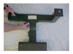
Take the tail beam and assemble securely to the flat mounting plate on the back of the seat assembly using four 8M nuts and 8M bolts.
