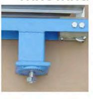
Insert 1 3/4" bolt into hexagon shaped opening, in the trap head carriage through the top of the pivot mount assembly; interlocking the gear mesh teeth. Secure with 1/2" nut using wrench.
