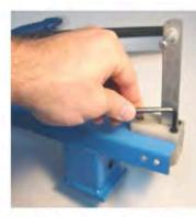
Attach Trigger by separating the 2 parts of the trigger block. Slide trigger facing up into slot in the back of the trap head with the small part of the block on top of the trap head and the large piece below. Tighten the bolts securely through the block using the nuts underneath.
