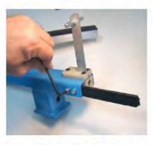
Attach handle to inside of trap head by screwing allen bolts through trap head into handle. Tighten securely.
