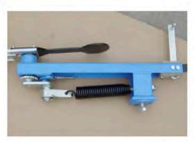
Rotate the arm counter clockwise into the 1 o'clock position. Hook the black main spring into the silver swiveling spring hook, which is attached underneath the throwing arm/clutch pivot point.
