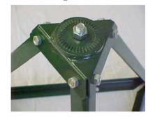
Take the 1 3/4" hex bolt and push up through the center hole of the Triangular/Top Pivot casting securing with the 1/2" hex nut. This is where you will attach the 3 Pivot Mount and your Trap Head.
