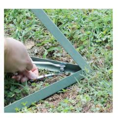
If the ground is soft you should also use sand bags or mount directly to a sheet of plywood. Make sure you control the trap by holding onto the handle when in use.
