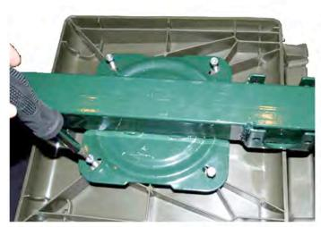
If not already attached, secure the seat to the seat post with the 4 self tapping screws.
