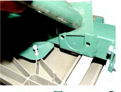
Take the four support legs and slot the into the leg brackets as per pictures. Note that the predrilled hole at the end of each leg are the feet not the mounting brackets. Therefore, The square plate with the hole should be the end that will be sitting on the ground. Now you're ready to attach the trap head. (separate instructions)
