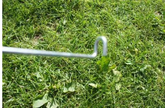
Supplied with the fox trap is a long metal rod with 2 hooks as shown in the photo, the U bend hook in the right photo hooks through the metal plate inside the trap, the hook to the left hooks onto the spring clip as shown in the below picture. The rod hooks onto the u bend spring clip whilst the L shape metal hook goes onto the door whilst in the cocked position.
