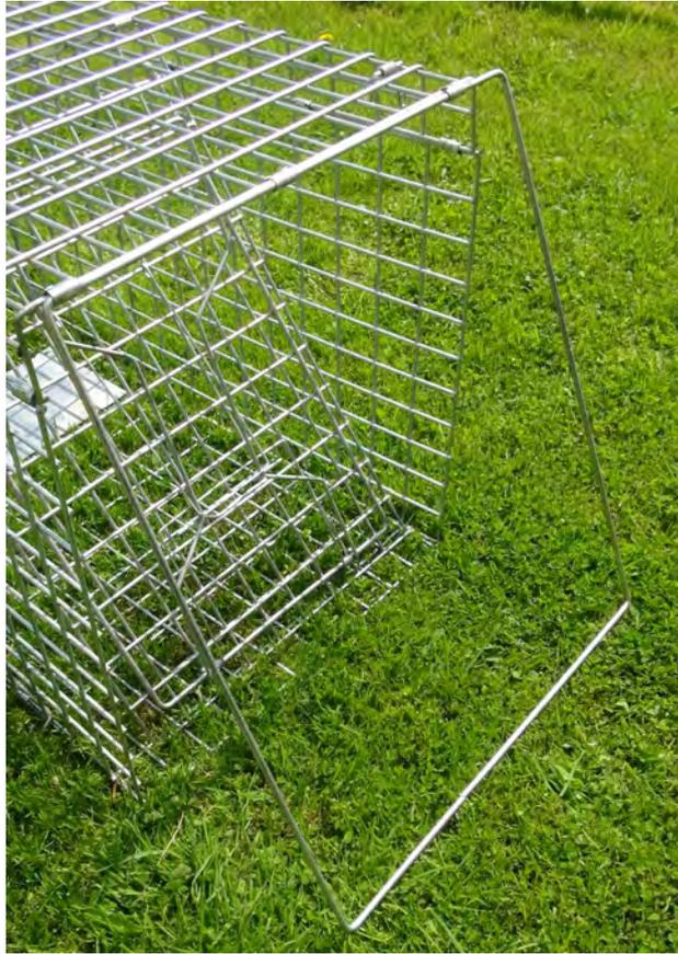
At the front and the middle of the trap there is a support bar which will stop the cage from folding. Fold the bar and tuck it under the base of the trap
