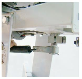
Rotate arm counter clockwise to 12:00. Insert Black Main Spring into silver swiveling spring hook. Attach Spade Bolt to spring & feed thru opening at back of trap. Tighten to show 1 or 2 threads on the back side of the lock nut. Now tighten the inner lock nut closer to the frame.
