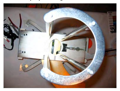
Safety Ring Guard shows the projection of the throwing arm when in use to ensure safety.
