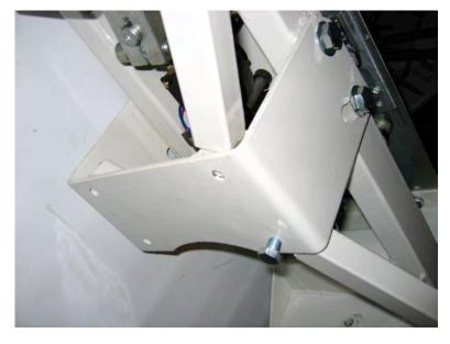
Attach each pole ensuring that the smaller poles are in the front of the trap and larger poles are in the rear. Now attach horseshoe to top of poles and tighten hex screws.
