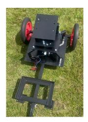
Mount the wobbler kit onto the trolley and align the predrilled holes. You may need to loosen the clamp bolts to align the holes.
