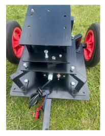
Once you locate 1 x bolt per foot, tighten each foot nut and bolt, then tighen each clamp bolt holding the leg on. Do not over tighten.
