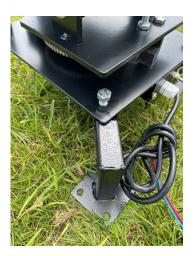
Attach the 4 x short legs onto the wobbler kit and nip the clamp bolt hand tight for now.
