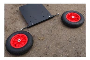
Slide the 2 x wheels onto the axle and fasten the m22 nylon nut onto the axle end thread.
