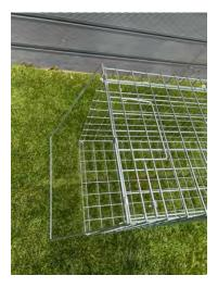
At the front of the trap there is a support bar which will stop the cage from folding. Fold the bar and tuck it underneath the base of the trap
