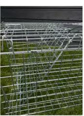
Attach the door on the 8th metal runner, normally indicated with red arrow stickers. The trap door should end so it is inside the cage as shown in the image to the far right. Use the ring clips provided to clamp the door to the roof of the trap. You can use a cable tie to hold the door whilst you attach the metal clips. Once fastened, the door will automatically be set in the trapped position.
